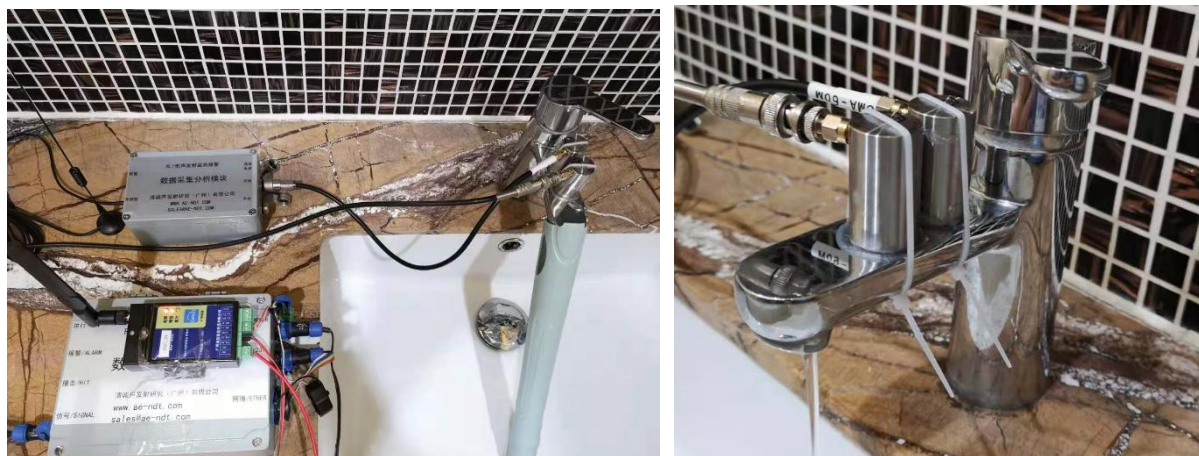
Fig 6 Layout of testing on tap and RAE1/RL1
